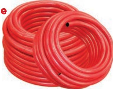
The hose is double layered with red cover and black lining. Material used for inner lining and cover of hose is plasticized PVC compound and high tensile textile polyester yarn is used for reinforcement of hose.
