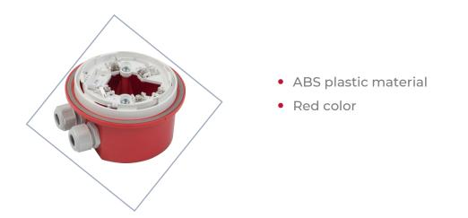
SensoIRIS WSB IP65 is a waterproof protected deep base specially designed for outdoor installations of analogue-addressable sounders SensoIRIS series. The deep base is suitable for wall mounting in applications in aggressive environments requiring IP65 protection of the devices. SensoIRIS WSB IP65 comes in a kit with a solid rubber gasket, o-ring sealant and IP65 rated cable glands. SensoIRIS B124 standard base is mounted with screws.
